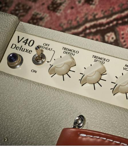
depth controls for the tremolo with level and tone controls for the valve-powered spring reverb. There are two small tonealtering mini toggle switches: Voice I/ Voice II swaps between a 'blackface'-type American EQ response and a slightly stronger midrange for more punch and drive, while Mid Kick is tied to the midrange pot and adds more focus.
