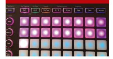
The modulation sequencer is a little simpler, with each step featuring just a level value to be sent to the mod matrix. Shift pressing 'Mod Seq' will smooth out the sequence, avoiding abrupt parameter jumps.
