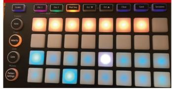
Inputting a sequence only via Osc 1 will cause both oscillators to follow the same pitch. As soon as seperate notes are added under Osc 2, the second oscillator will deviate and follow this new pitch.
