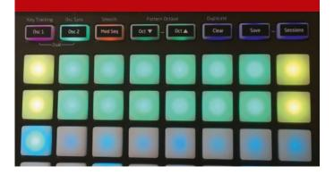
each individual pattern. This can allow us to create complex polyrhythms across the three quencer channels. For example, try a 16-step melodic sequence from osc 1, a 6-step pattern of notes on osc 2 and 12-step modulation sequence routed to the filter.
